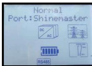
After pressing the "OK" key, the characters on the LCD begin to blink. Then use the down key or up key to select the Port: ShineMaster, and press OK to complete the setting
