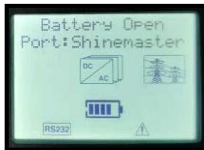
After pressing the "OK" key, the characters on the LCD begin to blink. Then use the down key or up key to select the Port: ShineMaster, and press OK to complete the setting
