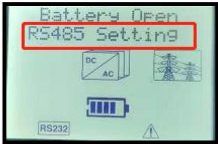
4.3. Press the OK key to enter the ShineMaster port selection screen. Select a port for SPH to communicate with ShineMaster.
