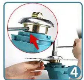
4. Snap the headstock with an allen key and tighten the nut with a socket.
