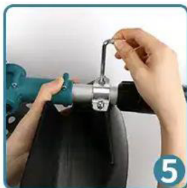
5. Installation of grass guards
