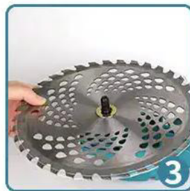
3. Installation of circular saw blades aligned with holes
