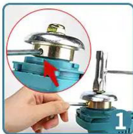
1. Snap the headstock with an allen key, unscrew the nut with a socket
