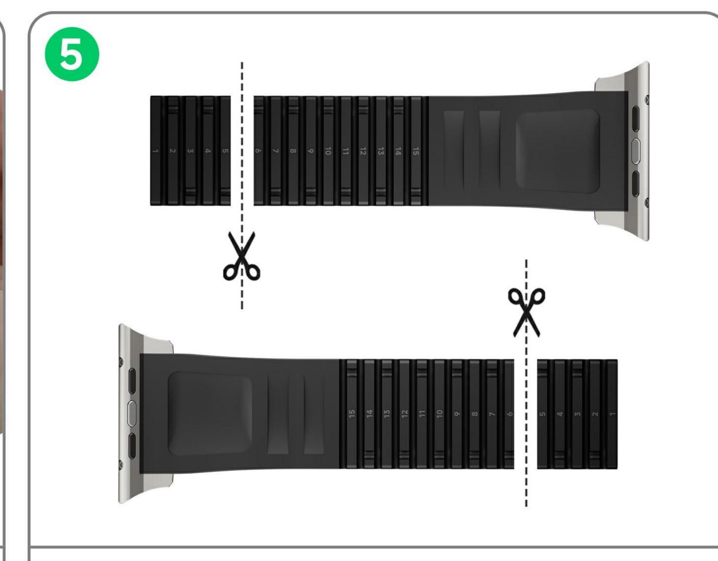
Use a utility knife or scissors to cut both straps at the pre-cut position
