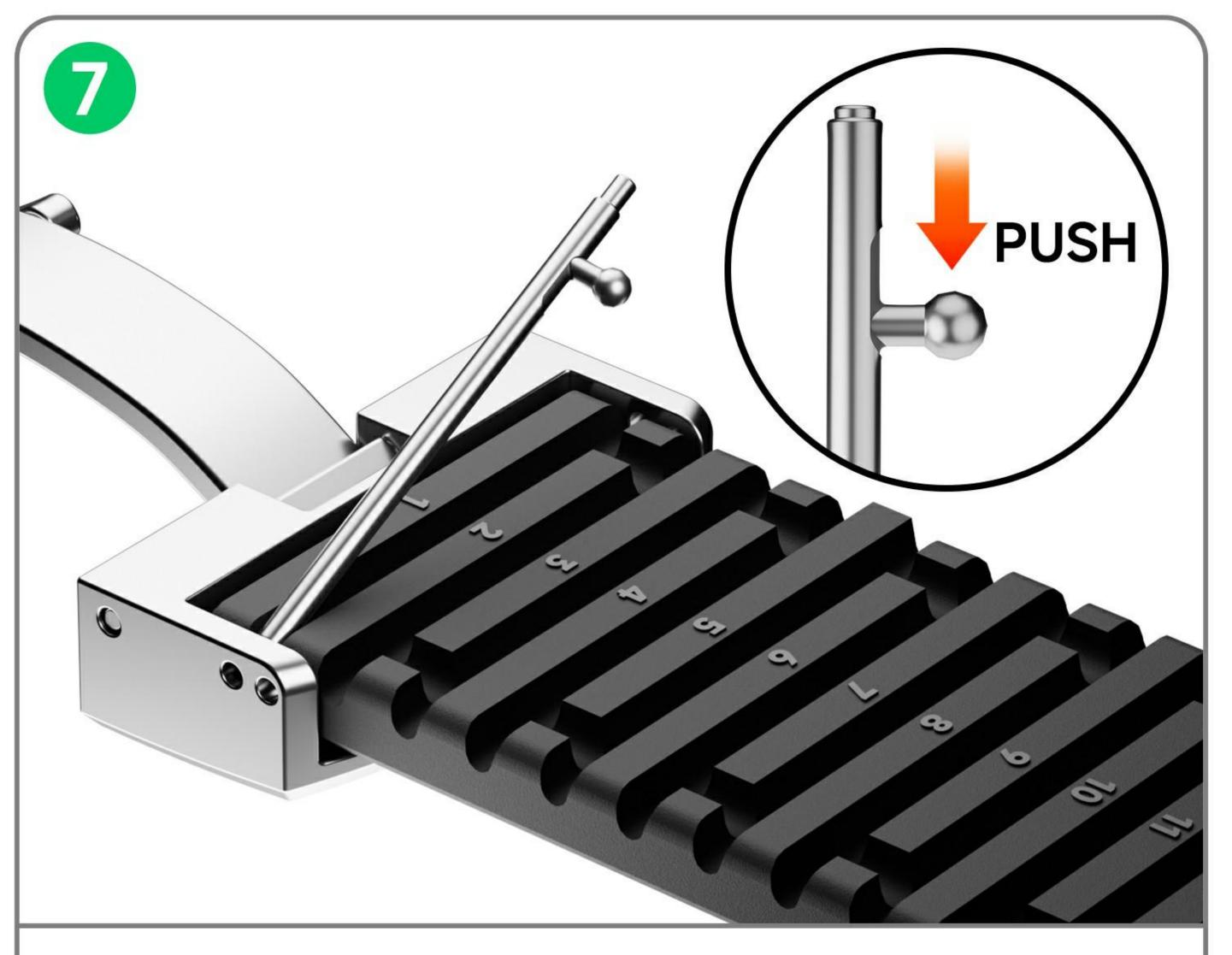
As shown in the picture, first insert one end of the pin into the watch buckle Then press the switch to install
