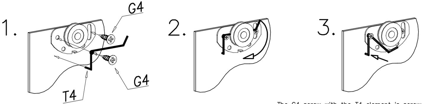
GB The G4 screw with the T4 element is screwed in so that there is a small clearance allowing the rollers to bend on the spring.
