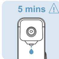
**5 mins** Flush (Make water purifier run) more than 5 mins after long time no use.
