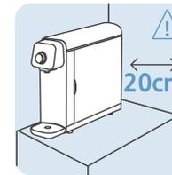
The back and sides of the product needs more than 20cm spaces apart from the wall for convenience of filter replacement. And do make distance between tap water and inlet of product NO more than 5m to connect water hose.
