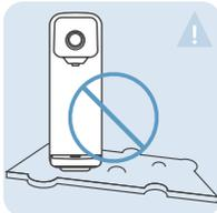
Do not install on uneven or inclined floor and do not put on sitting cushion, carpet, pallet and floor pad. It can cause not only damage and noise, but also injury to the user.
