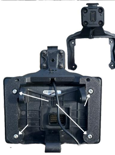
**4.** Unscrew bolt under the left side of the display.
