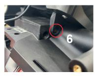
**6.** Unscrew 2 bolts holding the display bracket.
