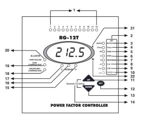
On the front panel of RG-T, there are warning lights, display and 3 buttons for settings.
