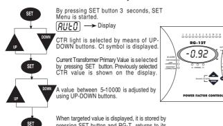
When targeted value is displayed, it is stored by pressing SET button and RG-T returns to its normal operating mode
