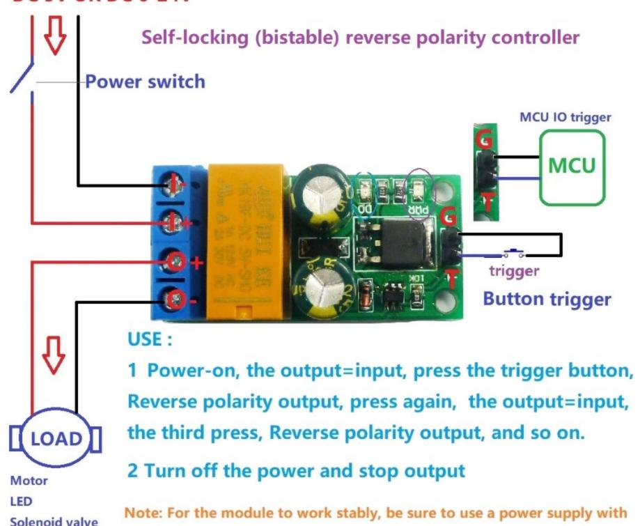
sufficient current. 3 times rated current required when motor starts
