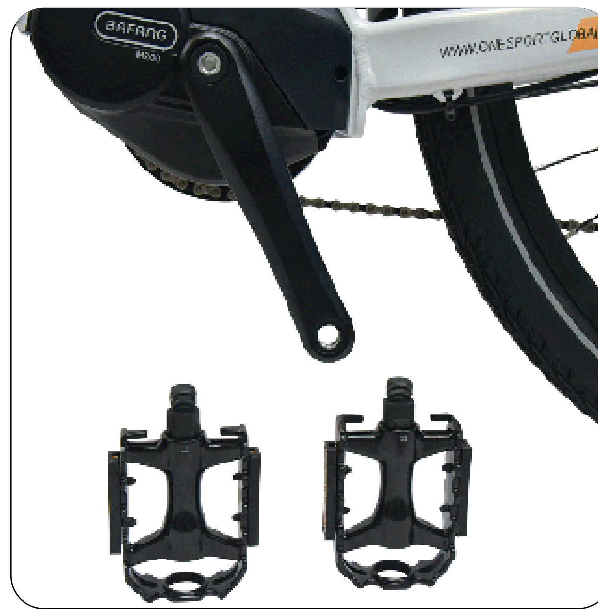
14. When installing the foot pedal, pay attention to distinguishing between "R" and "L".
