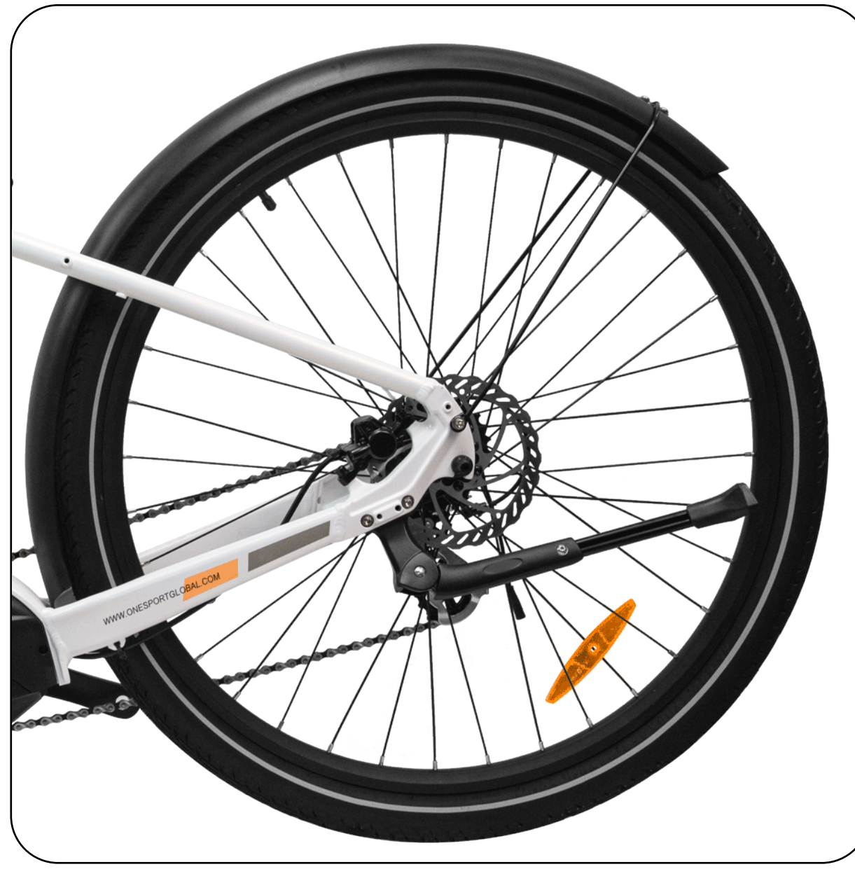
11. Install rear fender.
