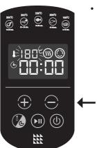
• To set to the temperature, use the (+) or (-) buttons – these will increase or decrease the temperature in 10°C increments from 80-200°C. You can press and hold the (+) or (-) buttons to skip quickly through the temperatures.
