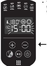
The control panel will illuminate and show the default temperature of 180°C. The default time of 15:00 minutes will be flashing.
