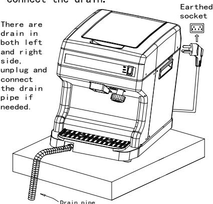
3. Lift up the cover and pour the ice cubes inside the hopper
