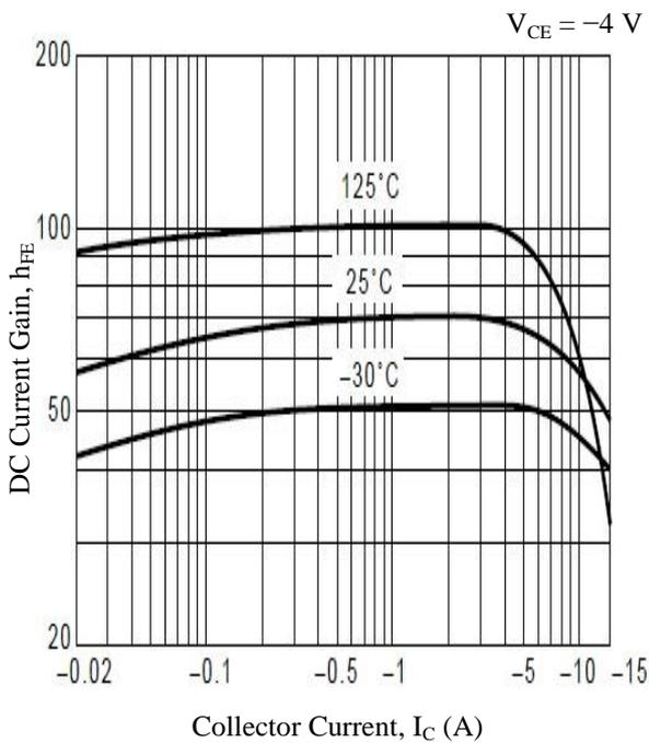
Figure 7. DC Current Gain vs. Collector Current
