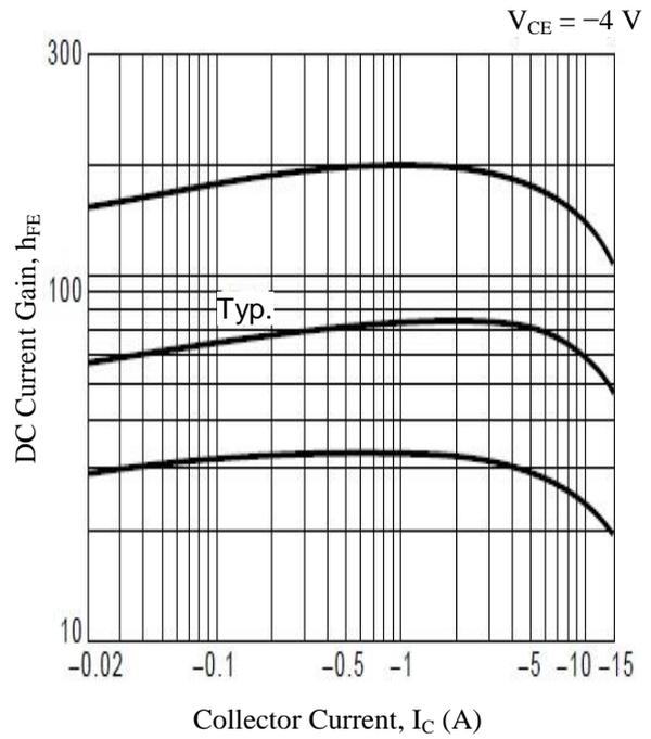
Figure 6. DC Current Gain Variation vs. Collector Current
