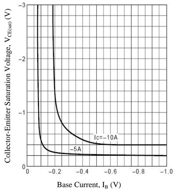
Figure 4. Collector-Emitter Saturation Voltage vs. Base Current
