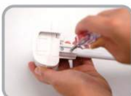
5.Drill the short screws into the iron tube with the phillips head screwdriver.
