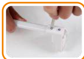
2.Drill the short screws into the iron tube with the philips head schroevendraaier.
