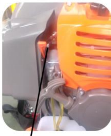
idle adjustment screw
