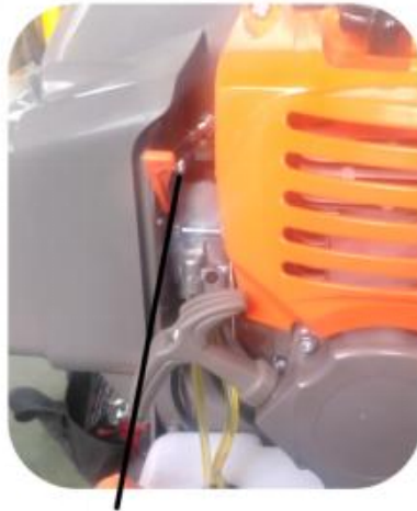
idle adjustment screw
