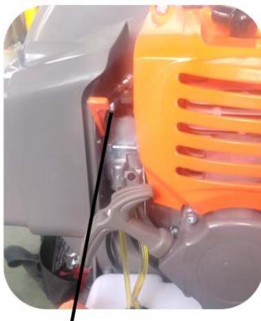
idle adjustment screw
