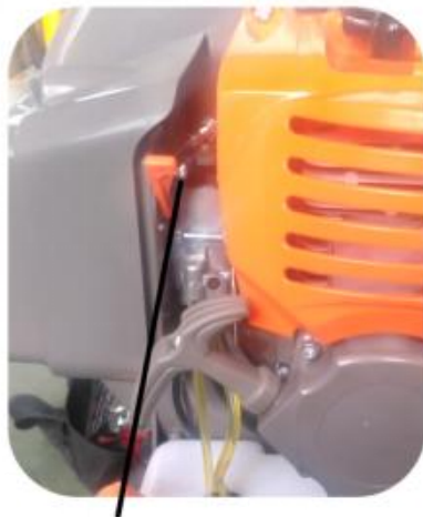
idle adjustment screw
