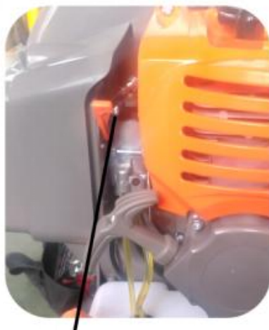
idle adjustment screw
