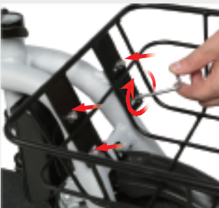
Tighten the four screws in the right direction
