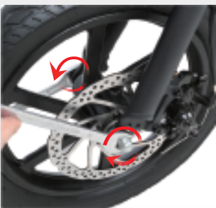
Fix the screws on both sides in the right direction
