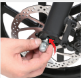
Place into the hole in the right direction
