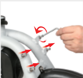
Loosen the four screws in the right direction
