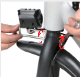
Fix the screws on both sides in the direction
