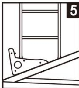
**ROOF JACK**-This position is valuable for leveling your ladder on a roof. Use only on an asphalt shingled roof and only up to a 7/12 pitch.(Shown here on a roof less than 5/12 pitch.(For roof pitches from 5/12 to 7/12, must be turned over and used similarly to the position shown in figure 1 above). For roofs steeper than 7/12 pitch, a RoofBoot (available from ProVisionTools, Inc.) or wooden block nailed to the roof to support the Ladder Tool is essential.
