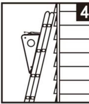
**LADDER JACK-**Position the Ladder Tool on ladder rung as shown here with plank leaning slightly into the ladder.In this position,the will accomodate a 2"x10"or 2"x12" wooden.
