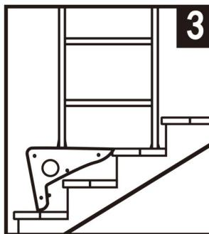
**STAIR STEPS-**The can be used on carpet,wood,concrete,brick or aggregate steps.Keep rear feet on lower step safely from edge of tread (at least 1") and in stable position on top tread as shown.
