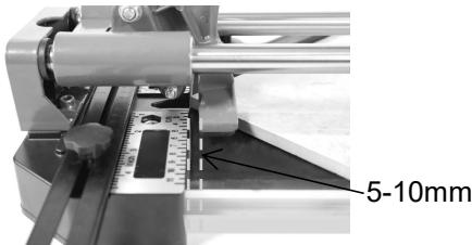
Tips: Do not put the tile too inside to make sure the scoring line is a whole line, after scoring, it is better to pull back the handle to let the breaker slightly backtrack 5-10mm, it's the best position to break the tile.
