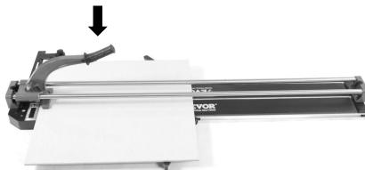
After scoring and without moving the tile position, the breaker is slightly in the front edge of the tile and front stop.
