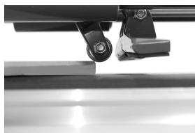
Slide the wheel forward by pushing the handle down with medium pressure.
