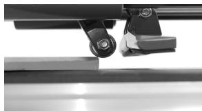
Place the cutting wheel on the rear edge of the tile.
