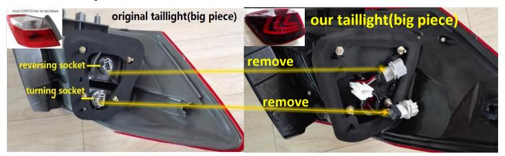
As for installation of big piece, remove your original sockets to install on our taillight wires for LX/Sport/EX model. The bulbs on original sockets may not be needed on our taillight(big piece), so you can remove the bulbs.
