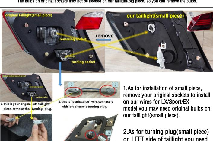
3.connect the plug and the wire 4. install this wire on our LEFT side taillight
