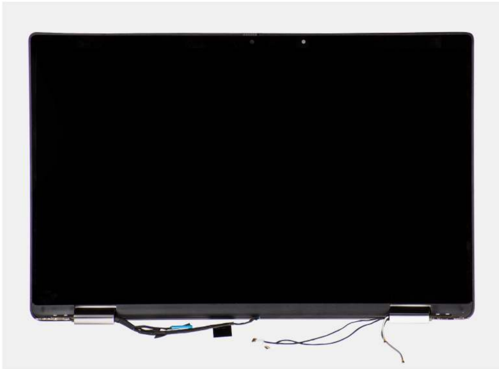
Figure 5. Display assembly with antennae cables
