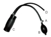
6.After test, pull off the smoke nozzle, release the inflated air by open the Pressure Relief Valve (A) next to the Hand Pump(B).
