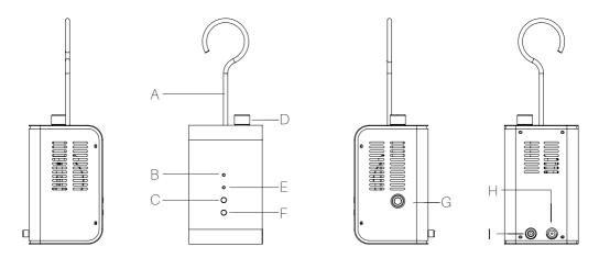
A-Hook, B- Power indicator, C- Run key, D- Fill port, E- Work air inport, F- Stop key, G- Level window, H- DC12v input, I-Smoke out port
