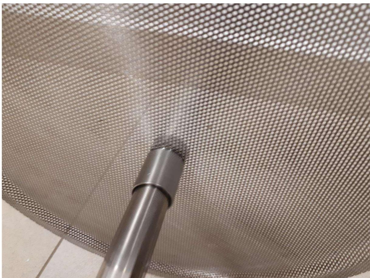
The sieve, assembled in this way, should be placed inside the cylinder that will be placed in the boiler, but before this, the top end on the tube should be unscrewed and plugged with a white plastic cap - the boiler will be ready to be filled with malt:
