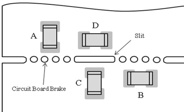
Stress strength according to the mounting position:
