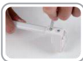
2. Drill the short screws into the iron tube with the philips head screwdriver.
