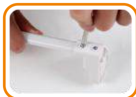
2.Drill the short screws into the iron tube with the philips head cacciavite.
