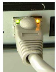
So, now look on the network switch for more LED indicators. You should see an illuminated LED for each connected port. You should therefore see illuminated LEDs for two ports – one for the connection to the laptop and one for connection to the counter. If you have other equipment connected to the hub then those LEDs may also be illuminated.
