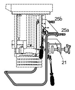
For applications near the ambient temperature, the cooling coil (order no. 8 970 105) must be connected to the water mains.
