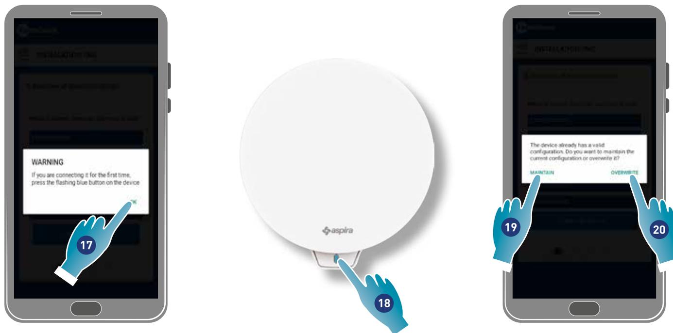
17. Touch to confirm and wait for the blue LED on the device to light up
