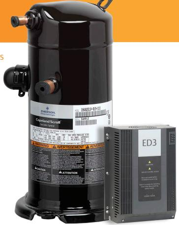
XHV qualification for A2L refrigerants (R454B/R542B) is expected for the end of 2018: the line-up will be the same as for R410A, but the compressors will be named YHV. The A2L class will have an impact on the PED class of the YHV compressors.
