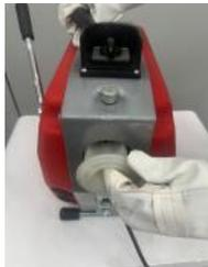
3. Pull the spring in the spring bin out about 10 inches, and then insert the spring into the machine from the end of the machine with a fixed hole, lift the pin of the spring bin parts, push the spring bin into the fuselage, drop the pin, turn the pin falls into the fixed hole of the machine.(as shown in the figure).
