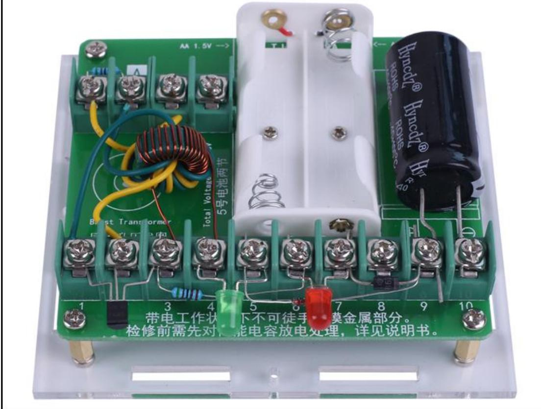
Step 21: Fixed 4pcs acrylic panels on the side by 4pcs M2\*10mm Screw and 4pcs M2 Nut.
