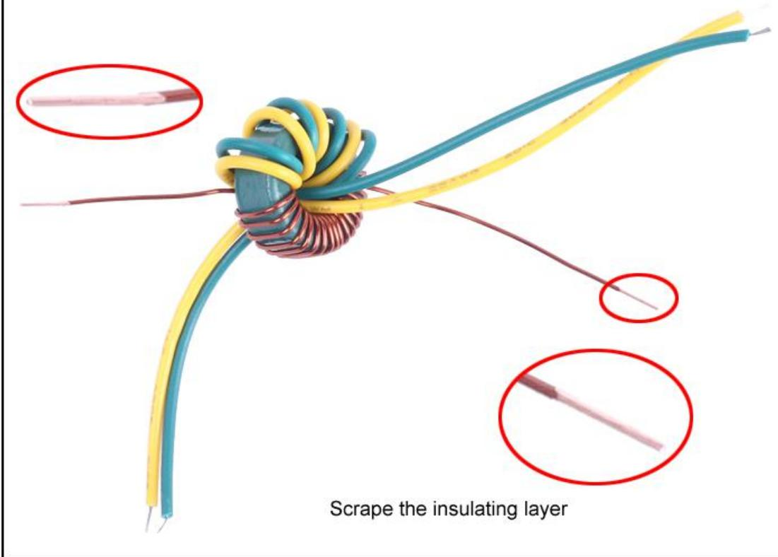
Step 10: Connect Magnetic Ring Coil. Note: As shown in the figure, the wires up the magnetic ring are connected to L1\*, L2\*, L3\* and the wires under the magnetic ring are connected to L1, L2, L3. Yellow wire connect to L1/L1\*. Green wire connect to L2/L2\*. Copper wire connect to L3/L3\*.
