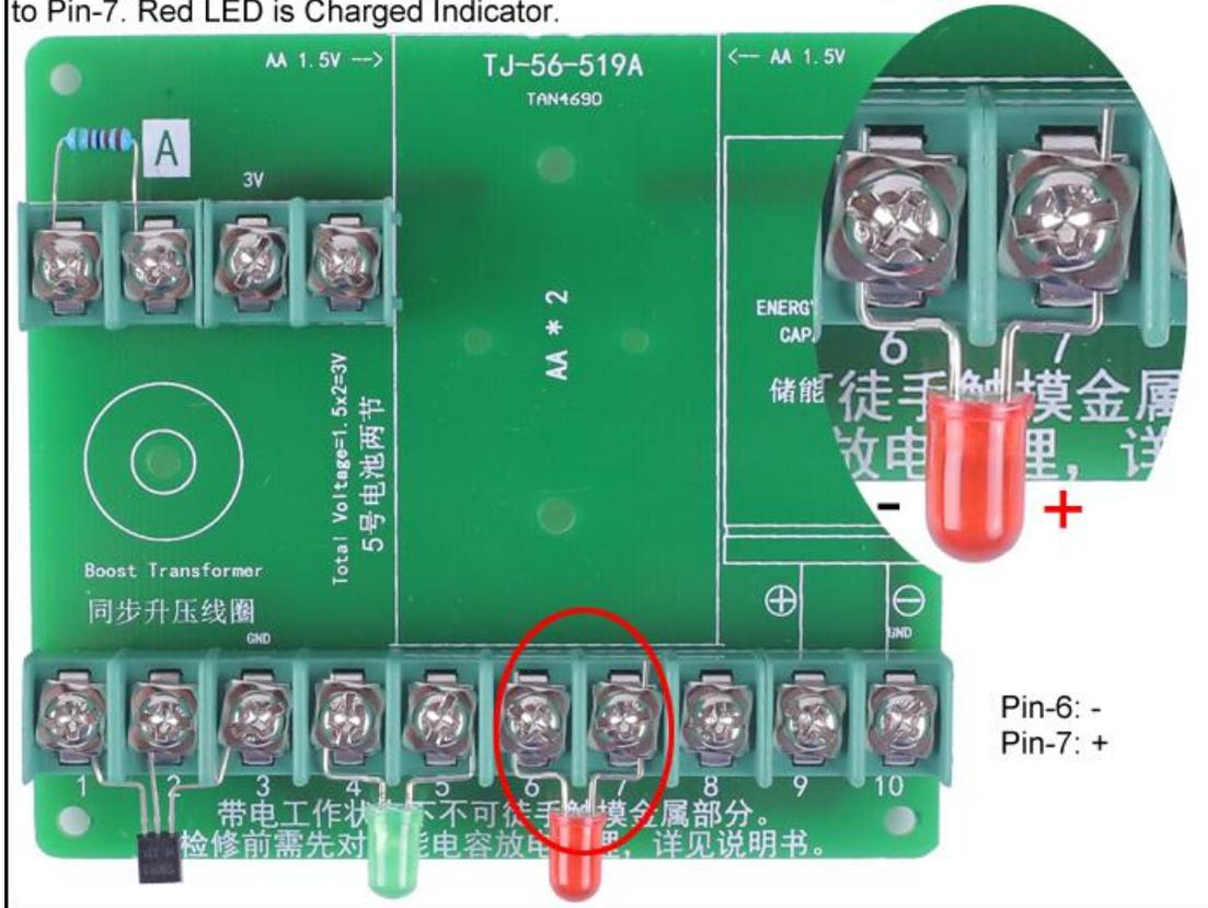
Step 6: Install 1pcs 5.1Kohm Metal Film Resistor at Pin-3 and Pin-6. Note that its pins should not be short-circuited with other components.
