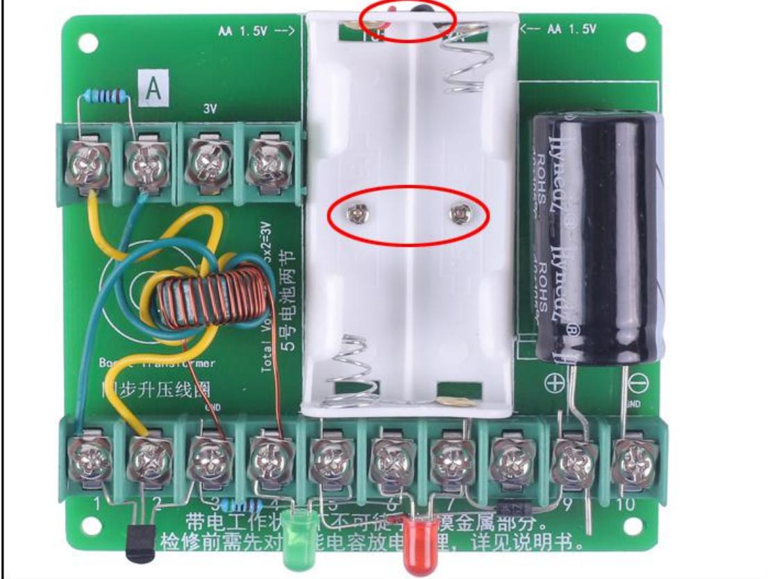
Step 13: Connect power wire form battery box to PCB. Red wire connect to '3V+' and black wire connect to '3V-'. User can cut excess wires.
