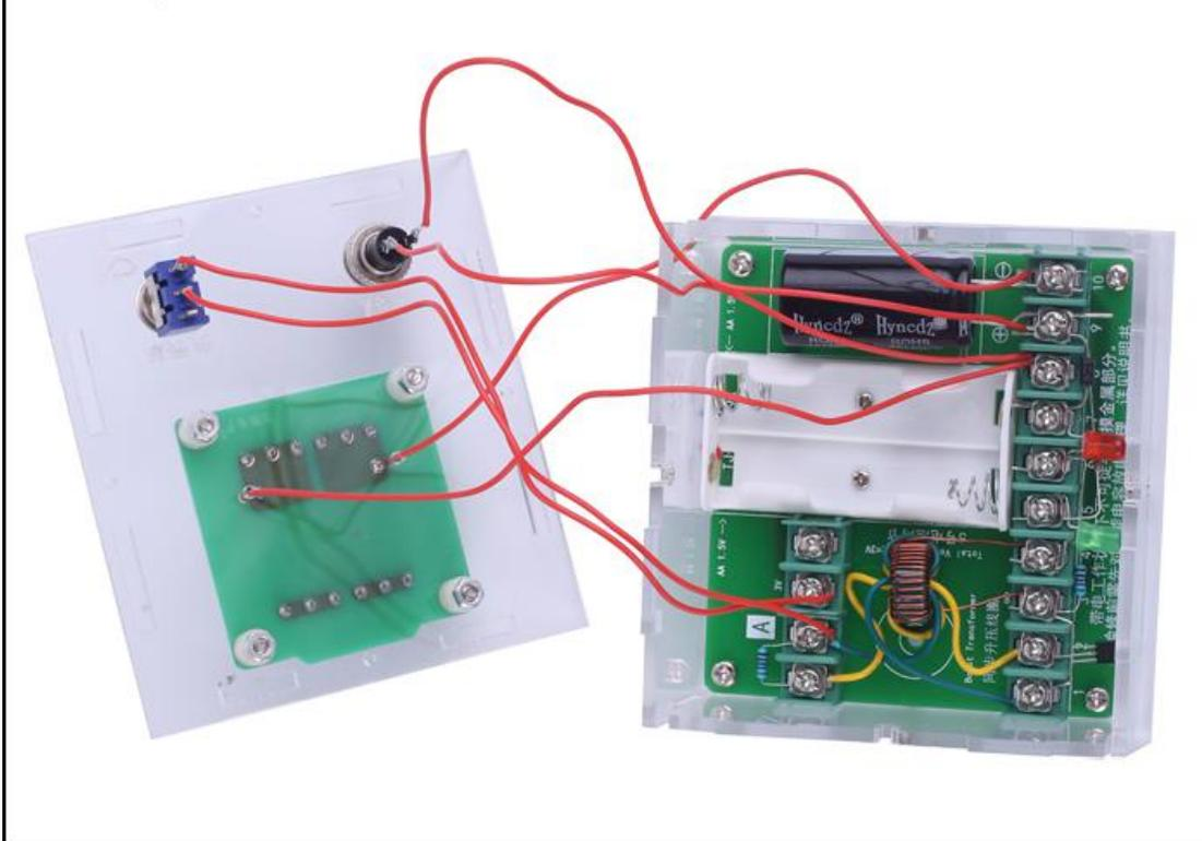
Step 25: Fixed the top acrylic plate by 4pcs M3\*6mm Screw. Note: Install 2pcs brand new AA batteries.
