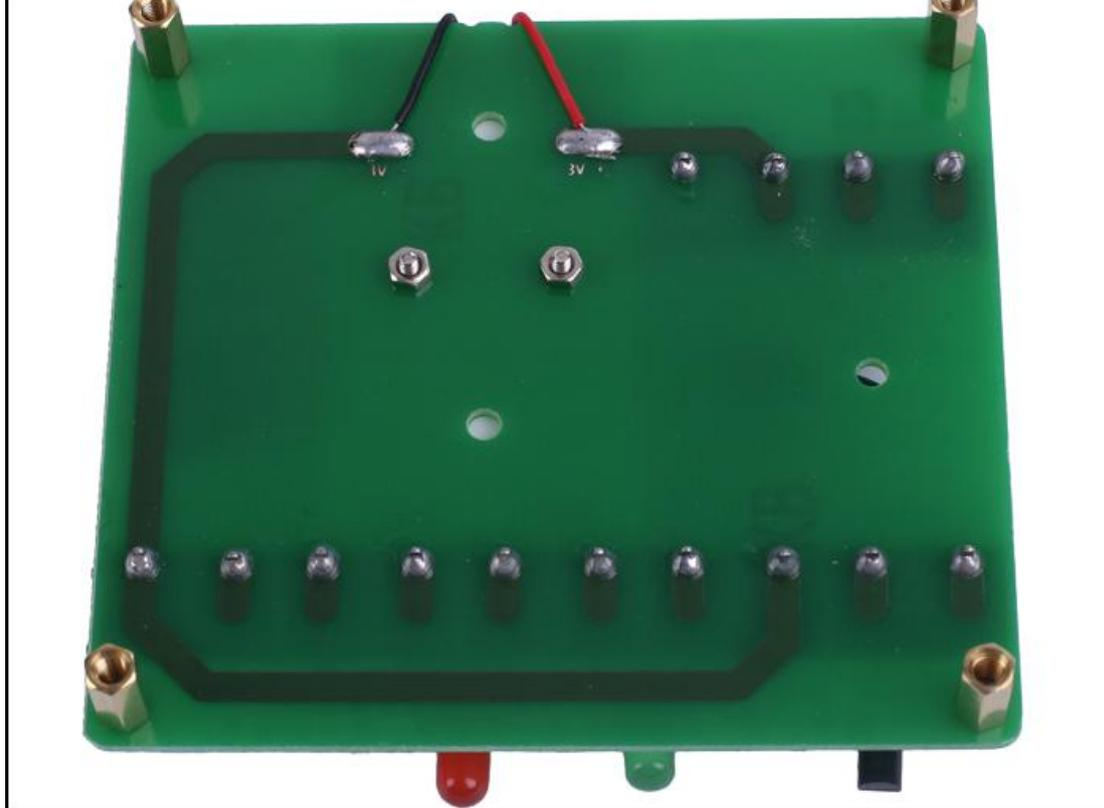
Step 15: Install 2pcs 20cm red wires on Smaller PCB.
