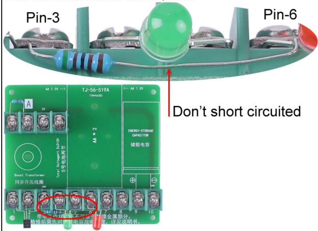
Step 7: Install 1pcs DO-35 1N4148 Diode at Pin-5 and Pin-9. Negative pole (Black marked) connect to Pin-9. Note that its pins should not be short-circuited with other components.
