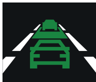
3. warning about the beginning of movement of an object ahead
