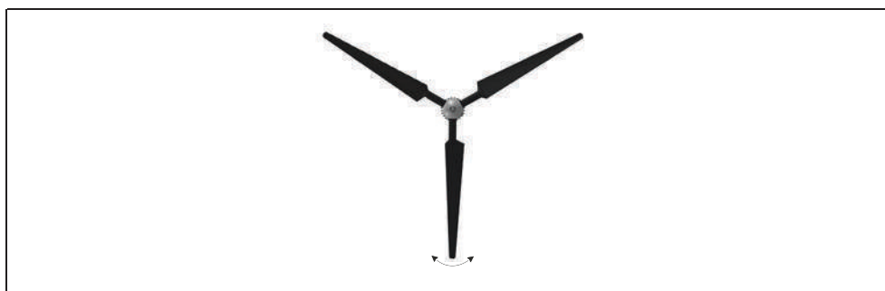
Fig. 7: Balancing the rotor (Y position)
