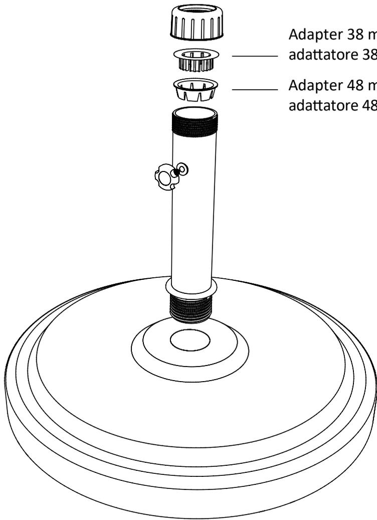
Adapter 38 mm / adapter 38mm / adaptateur 38mm / adapter 38 mm
