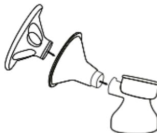
Install the silicone horn into the breast shield.
