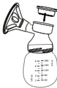
**Snap the silicone diaphragm into the breast shield.(As shown in Figure 3).**
