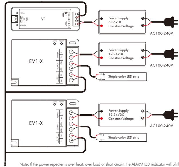
Note: If the power repeater is over heat, over load or short circuit, the ALARM LED indicator will blink.
