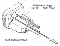
2 Turns (cw) will rise the threshold by one pressure decade. The upper threshold is 10% higher (hysteresis).
