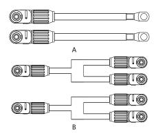
Anderson connector is used on the DC input side of the battery energy storage system. The specific connections are as follows:
