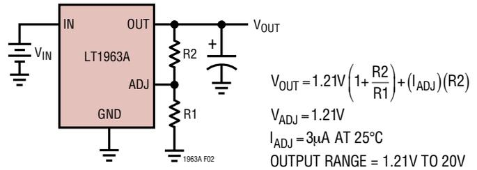
Figure 2. Adjustable Operation
