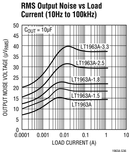
LT1963A-3.3 10Hz to 100kHz Output Noise
