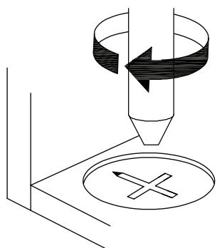
**EN** Turn cam lock clockwise to tighten.
