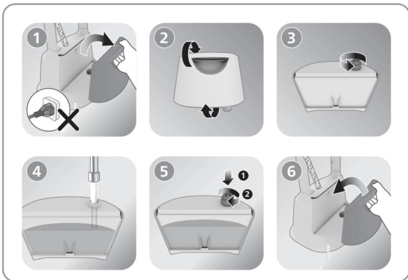
**EN** The appliance is suitable to be used with tap water. However, if you live in an area with hard water, we recommend that you mix an equal amount of tap water with distilled or demineralized water. This will prevent fast scale build up and prolong the lifetime of the appliance.
