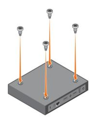
2 Attaching the client—Install the thin client on the P-series mount with the M4.07-6 screws included in the tool kit.
