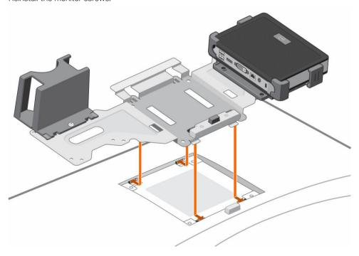
4 **Reinstalling the monitor stand**—Insert the upper stand tabs into the dedicated space on the P-series mount and gently press down until the quick release button snaps into place. Place the monitor in the upright position.
