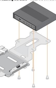
1 NOTE: The power button should face outwards and air vents should be on top end for proper heat dissipation.
