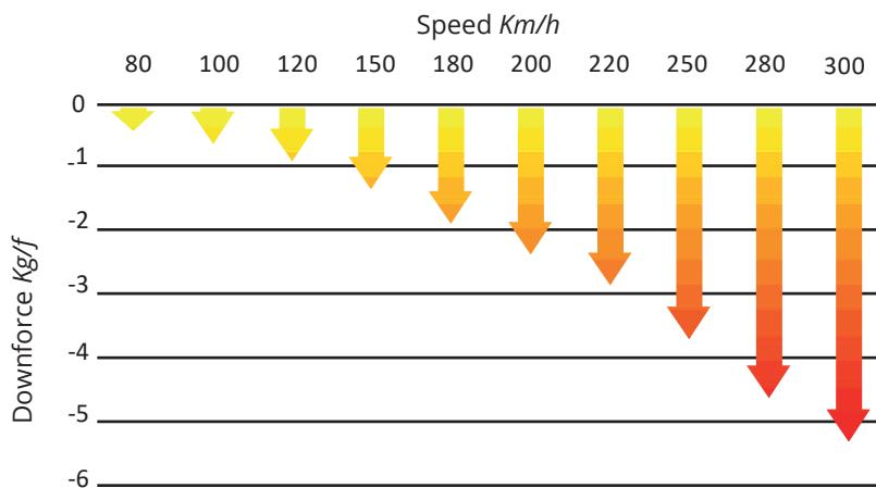
The Downforce that the spoilers generates raises potentially as the speed increases, at 200 km/h we get 2,4 Kg/f.
