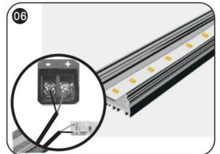
○ Connect strip wires to the output terminal of power supply, and dispose with waterproof, insulation, short-circuit and anti-corrosion protection at both the wire joints and the cut section of your strip (if any)
