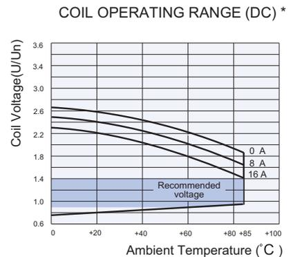
**Notes:** \* The use of a relay with an energising voltage other than the rated coil voltage may lead to reduced electrical life. An energising voltage over the above range may damage the insulation of relay coil.
