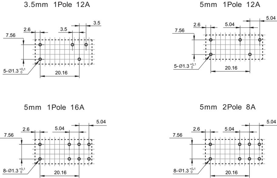
Remark: 1) In case of no tolerance shown in outline dimension: outline dimension  $\leq 1$ mm, tolerance should be  $\pm 0.2$ mm; outline dimension  $> 1$ mm and  $\leq 5$ mm, tolerance should be  $\pm 0.3$ mm; outline dimension  $> 5$ mm, tolerance should be  $\pm 0.4$ mm.
