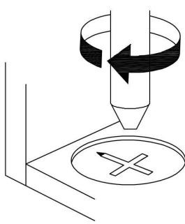
**EN**\_Turn cam lock clockwise to tighten.
