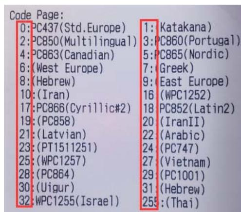
Input the desired parameter value in “Set code page”, and then complete the setting by clicking "set code page" button. Click "print code page" button to view the setup code.
