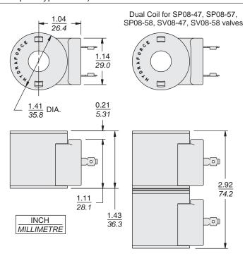
**EG**IP65 Rated 08-Size Coil; DIN 43650 Connector
