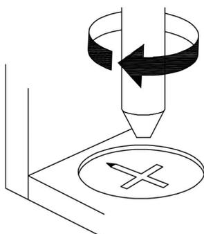
**EN\_**Turn cam lock clockwise to tighten.
