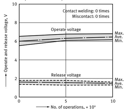
7-2. Electrical life test for wiper load (Motor free)
