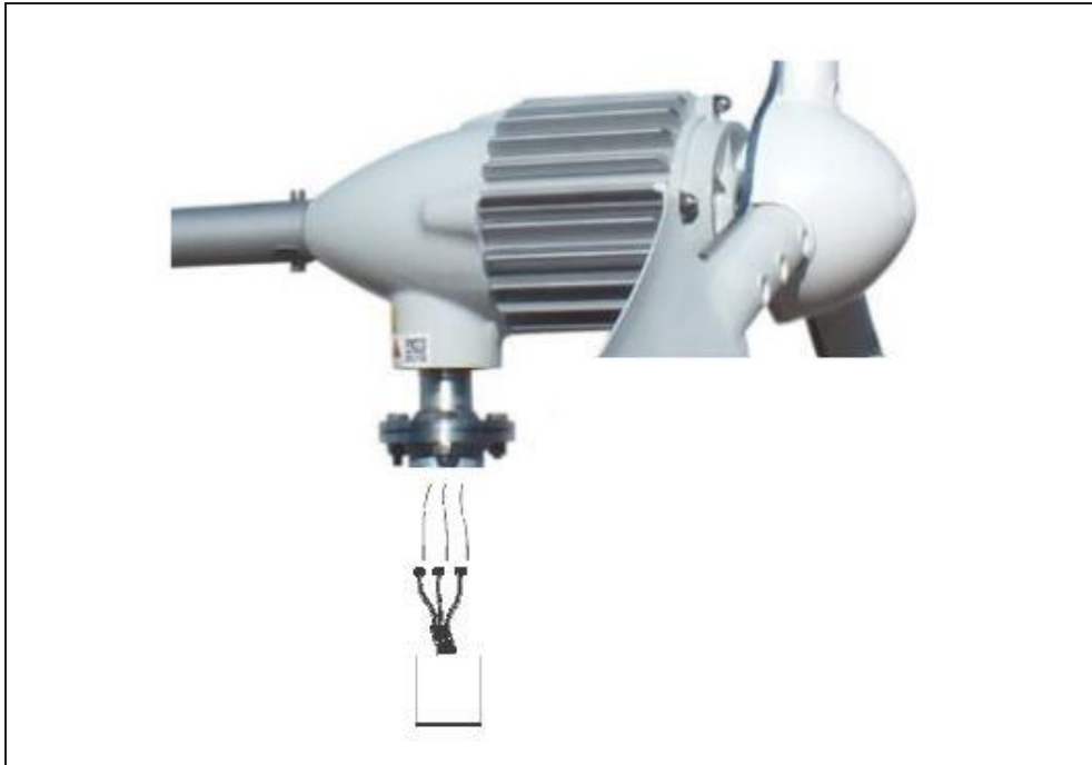
Fig. 8: Connecting the three-wire cable to the generator
