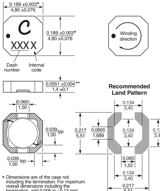
\* Dimensions are of the case not including the termination. For maximum overall dimensions including the termination, add 0.005 in / 0.13 mm.
